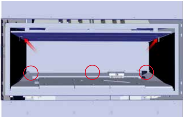
Panel Clip and Burner Tray Screw Locations
